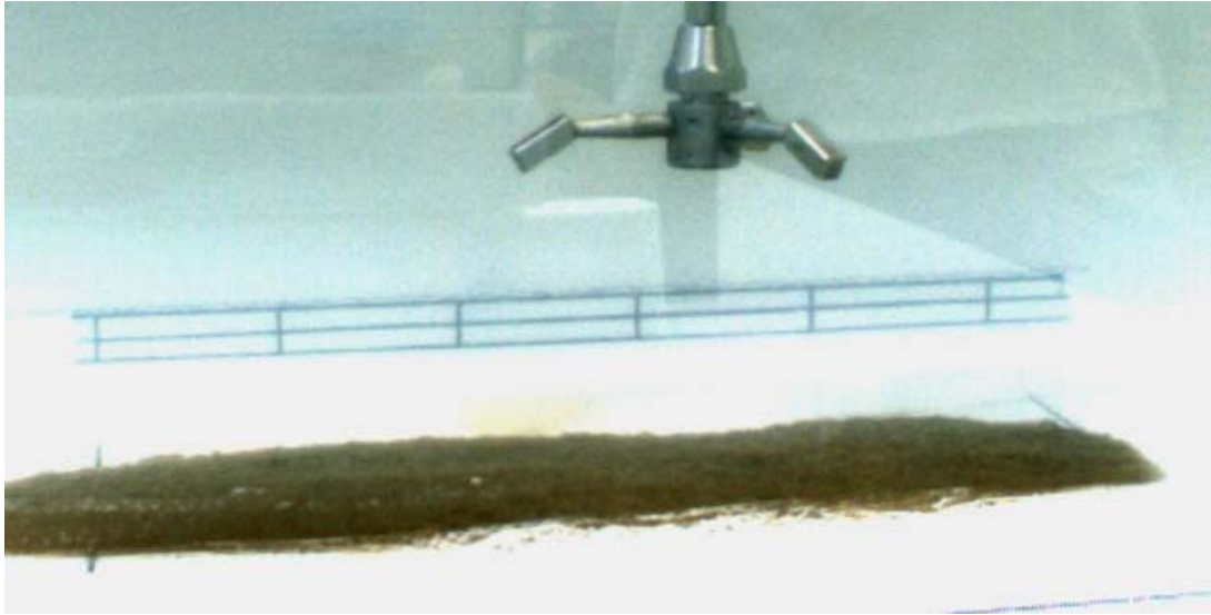
Floc mat at start of test
