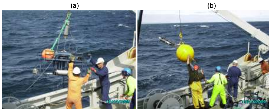
Figure 7: Photographs of second deployment of moorings in Bass Strait. (a) is a sea bed frame containing a current and wave meter, battery packs and LISST sediment analysers. (b) is a sub-surface buoy with a temperature and turbidity sensor mounted above. The two components shown are connected with a chain equipped with an anchor, multiple temperature sensors and an additional CM-04 current meter. Retrieval was achieved by the use of an auto-release mechanism whereby the main uplift buoy rises to the surface when the main anchor is jettisoned.
