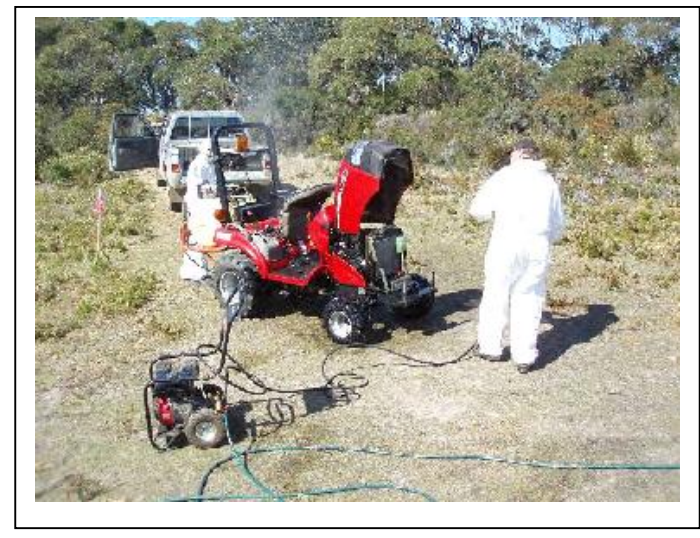
Portable high pressure water washdown of machinery
