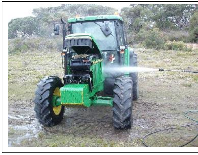
Portable high pressure water washdown of machinery
